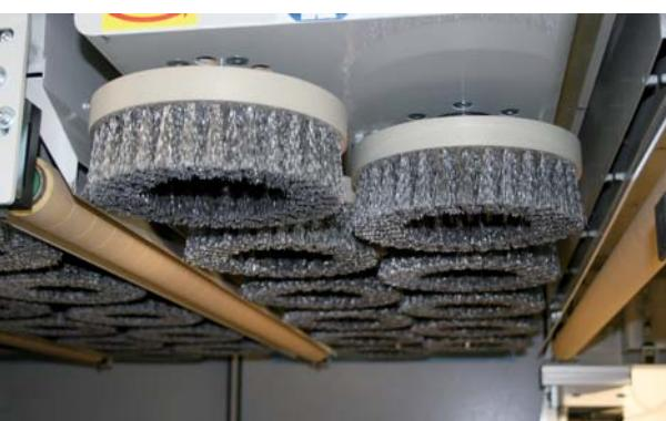
**The orbital planetary group allows to obtain a finish of excellence even when the grain of the wood occurs in different directions**
