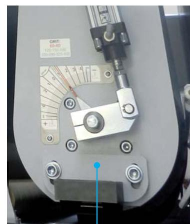
**Automatic pneumatic locking system counter support for de units**
