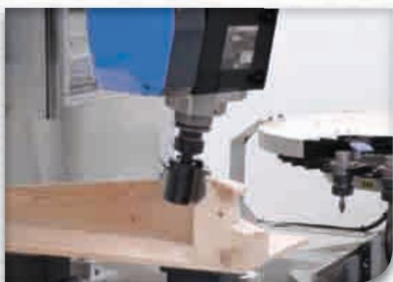
Liquid cooled electrospindle.
