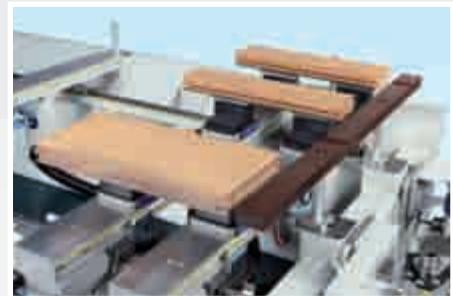
The side stop bar allows you to place multiple pieces without waste of time (to move reference stops) and money (additional stops).
