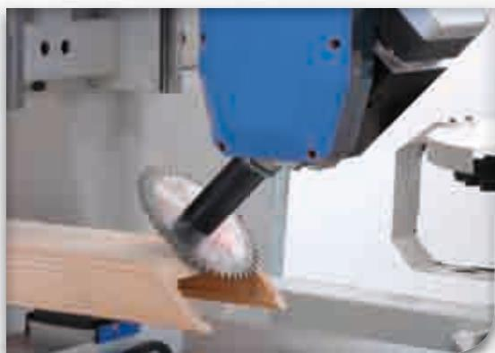
Routing unit with double rotation for 5 axis machining.
