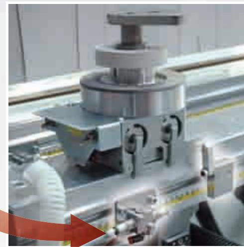
Mechanical clamping systems for solid wood, linear and arched components machining.
