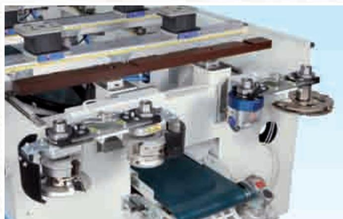
Automatic tools magazine on carriage side, tools magazine beside the router (Project 365) and tools magazine on the R/H side of the machine for bigger diameter tools.
