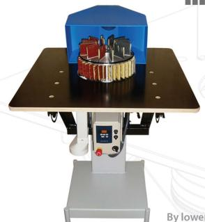
The Unosand multi disc is an adaptable machine ideally suited to component processing and the kitchen door industry for fascias and drawer fronts. By simply adjusting the speed and rotating the heads clock and counter clockwise, components can be prepared prior to paint or lacquer and perfectly denibbed between coats without the need to change abrasives.
