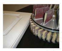
With the sanding unit lowered for fascia sanding the dust is extracted below the table.
