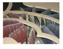
Disc sanding unit 250mm diameter with 24 keyways. A comprehensive selection of abrasive strips enables even the most complicated product to be sanded.
