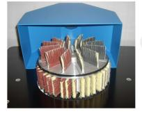
A simple extraction hood rests comfortably on the table top and can be positioned to assist with extraction when the unit is in edge sanding mode.
