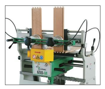
The milling cycle is obtained by gripping the two levers on the sides of the head and copying the contour of the previously adjusted template. This machine can process single male workpieces, single female workpieces as well as combined male-female workpieces.
